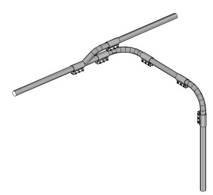
Figure 24: Modified Single-Line Y-Tube Installation
